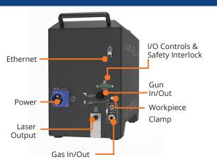
Clearly labeled rear connections make getting started fast and easy. Laser delivery, gas and gun control is pre-wired in a 5 m (optional 10 m) cable. Just plug in the power cord and gas connection, attach the clamp to your work surface and you are ready to go. An ethernet connection provides access to advanced parameter settings to fine tune and save process parameters.
